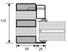
Standard profile with rubber beading (internal application)
