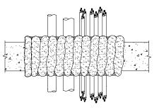
Example of P4 fire pillows sealing electrical cables and copper or ferrous pipes, in a floor penetration
