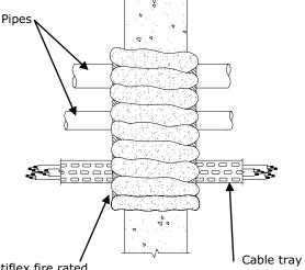
Multiflex fire rated sealant
