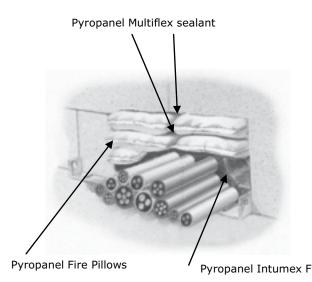
Example of P4 fire pillows sealing electrical cables and copper or ferrous pipes, in a wall penetration with Pyropanel Multiflex fire rated acrylic sealant and Pyropanel Intumex F
