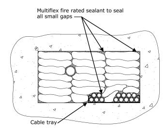
Typical elevation view of wall
