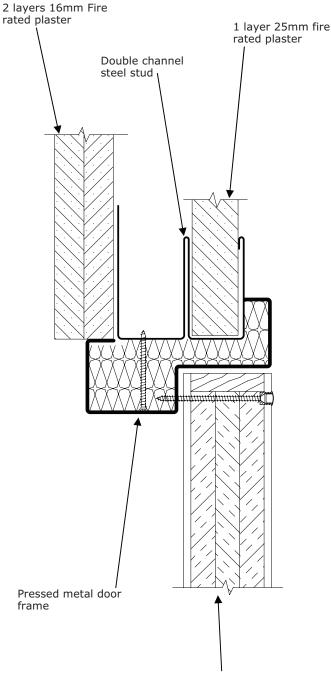
48mm Lift shaft wall access panel
