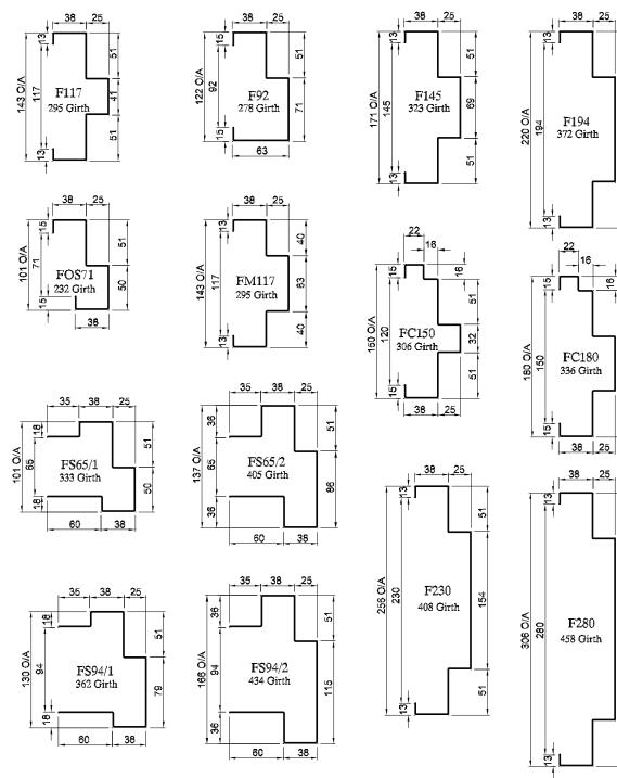
**Note:** When installed with appropriate door leaf, frames are fire rated up to 4 hours in masonry walls, and 2 hours in dry wall. Custom frame profiles available on request. Frames are typically 1.2-1.6 zincanneal unless otherwise requested.
